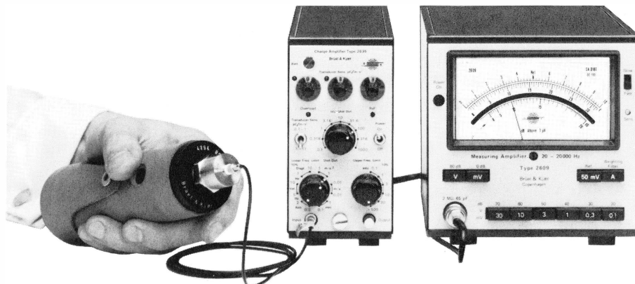
Fig. 2.4. Calibration of vibration measurement system
