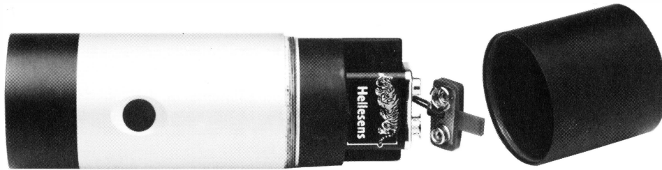
Fig. 2.2. 9 V Battery installed in the Calibrator
